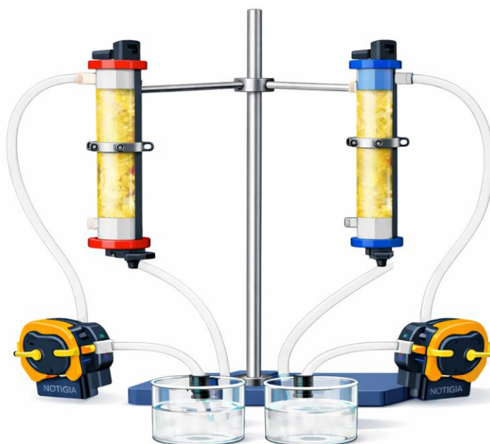
Figure 1. Schematic representation of the laboratory-scale ion-exchange column system
